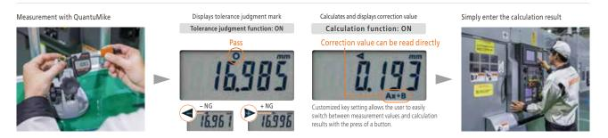
The micrometer determines whether the measurement value is within the upper and lower limits of tolerance and displays a tolerance judgment mark. The user can judge pass/ failure at a glance.
