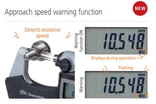
The approach speed warning function detects collisions with workpieces due to excessive speed. Even inexperienced workers can obtain stable and accurate measurement results.
