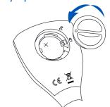
To change the CR2032 Li-ion battery, turn the battery cover located on the back of the meter counterclockwise to unlock. Remove cover and replace with + side facina up.
