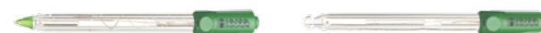
HI10530 Triple ceramic, double junction, glass body, refillable pH electrode with conical tip and temperature sensor Recommended for fats, creams, soil and low conductivity samples
