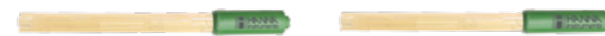
HI12300 Single ceramic, double junction, gel filled, PEI body, pH electrode with temperature sensor Recommended for field applications
