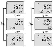
The average mode will calculate the average for a period of up to 24 hours. If a different mode is selected for that channel, the average will no longer calculate and the value will be lost.
