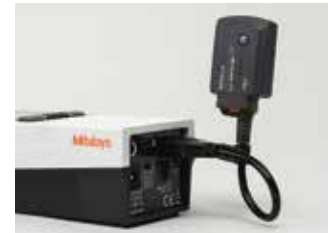
Example of the connection with SJ-210
