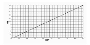
Fig. 5 W-20 Series Hardness Conversion Curve
