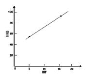
Fig. 9 W-B92 Series Hardness Conversion Curve
