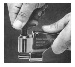
Fig.3 Regulate the adjusting screw
