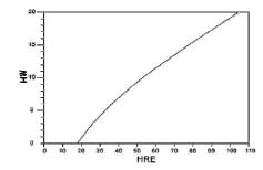
Fig. 8 W-BB75 Series Hardness Conversion Curve
