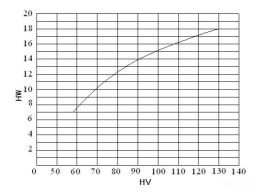
Fig. 6 W-20 Series Hardness Conversion Curve
