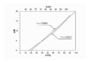
Fig. 7 W-B75 Series Hardness Conversion Curve
