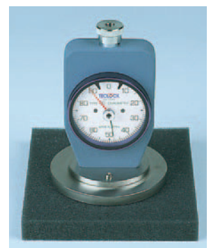
Hardness measurement of sponge sheet with GS-744G. Judge of dispersibility of foam measure
