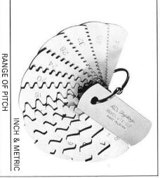
6, 7, 8, 9, 1 26, 28, 30, 6, 7, 8, 9, 10, 11, 12, 14, 16, 18 per inch 3.5 3.75 4.0 4.5 5mm 3.25 3.5 3.75 4.0 4.5 5mm 2 2·1/2 3 3·1/2 4 4·1/2 5 per inch 2 2·1/2 3 3·1/2 4 4·1/2 5 per inch .5 .75 1.0 1.25 1.5 1.75 2 2.25 2.5 2.75 .5 .75 1.0 1.25 1.5 2 2.25 2.5 7 8 9 10 11 12mm Φ 9 10, 11, 12, 14, 16, 18, 20, 22, 24, 32, 36, 40, 48, 64, 80 per inch 7 12mm 2.75 3 3.25
