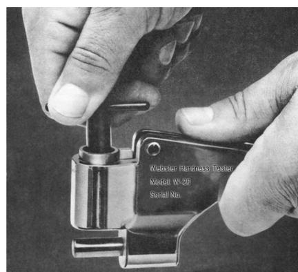
Fig.4 Regulate the adjusting nut
