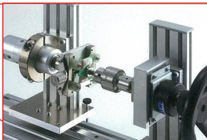
Torque-Angle Measurement of a small switch
