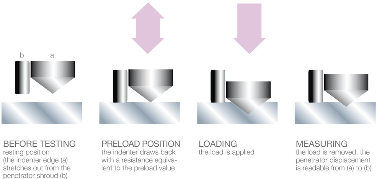
This new system makes use of the characteristics of an elastic component, which from load at zero progressively reaches the maximum load and then returns to zero. This component is previously compressed, and then during testing it acts on the penetrator. Thanks to this method, the test load is definite, as it is not produced by an impact but given by the characteristics of the elastic component. In this way, the test result is not influenced by any deflection of the work piece.
